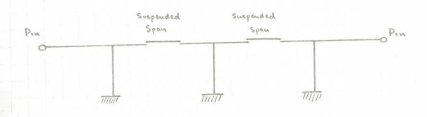
form of foot bridge envisaged, with very light sections and of Suspended span and contilever construction would be susceptible to unpopular and possibly deleterious vibrations. After consultation with the R.R.L., various Research pamphlets, and after visiting other bridges of a similar construction that have been built, the following measures were taken:
