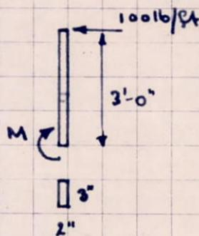
$$\text{Stresses, } \sigma = \pm \frac{21,600}{0.993} = \pm \underline{\underline{21,800 \text{ p.s.i.}}} \quad - \text{O.K.}$$
